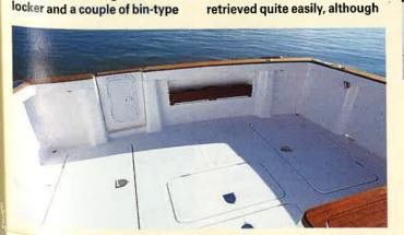
the wings of the compartment are occupied by the water tanks. On the down side there is no false bottom to keep things clear of the bilge, and we would have preferred to see the steering gear boxed in so that the rudder stocks cannot be fouled.
