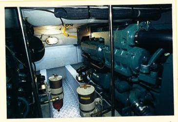
servicing, there is sufficient room right over and around the engines to get at the necessary filters and belts without troubling to get any more of the sole raised. This is a good thing because, although it is possible to take up more of the sole, it comprises not loose panels but a sizeable moulding that requires some perseverance to free.
