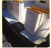
return if you are boarding from alongside. It would have been nice to find a helping handrail. but in fairness the builders have tried to keep the wood-protected coamings as clear of obstructions as possible so as not to tangle any fishing gear. To this end, for example, the stern cleats are of the pop-up variety.
