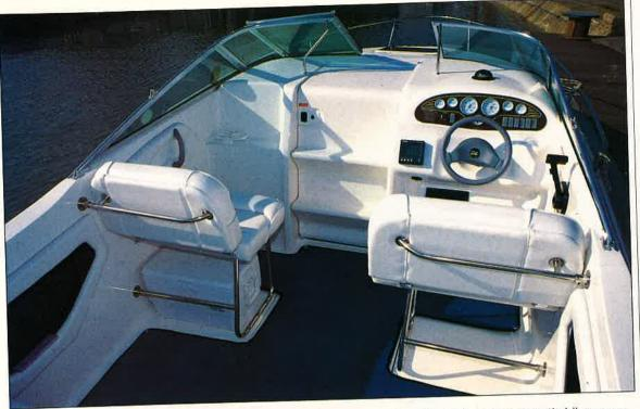
Left: the helm position is comfortably laid out, whether you prefer to sit or stand, although the twin seats are wide singles rather than genuine doubles. Below: the engineroom is neatly arranged, but the transom bench which covers the access would be easier to lift if attached with hinges.
