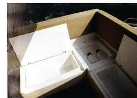
Lined lockers and bilge pump access points
