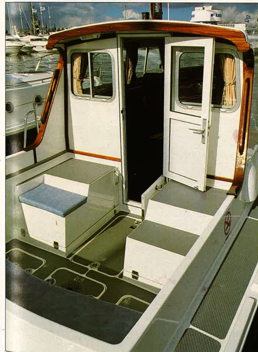
Left: Seaward's version of the Nelson 28/29 has ample headroom and space to walk through the saloon. Above: the settee's backrest hinges up to create twin bunk-berths (above). Above right: forward are a galley and double cabin. Right: cockpit seating is provided by a transom bench and the engineboxes.
