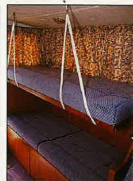
Left: Seaward's version of the Nelson 28/29 has ample headroom and space to walk through the saloon. Above: the settee's backrest hinges up to create twin bunk-berths (above). Above right: forward are a galley and double cabin. Right: cockpit seating is provided by a transom bench and the engineboxes.
