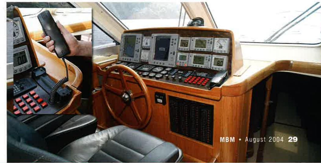
below The inside helm has space for two of everything, and the VHF handset's cord is self-parking.
