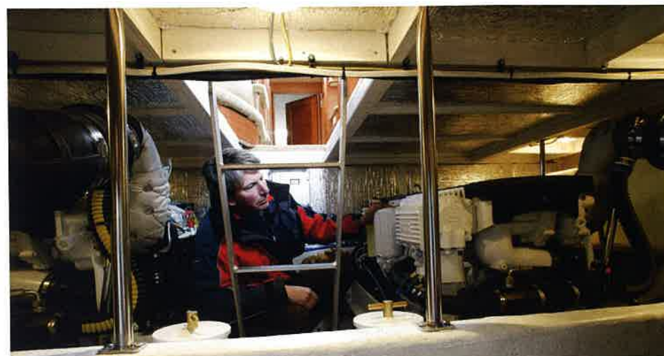
Access to the twin diesels is best achieved through a lift-out hatch in the saloon sole
