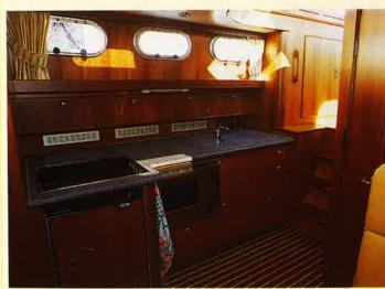
return housing the hob and fridge. Disappointingly, bearing in mind the fastidiousness of the builders elsewhere on the boat, this has no fiddles, a point which could easily be remedied.
