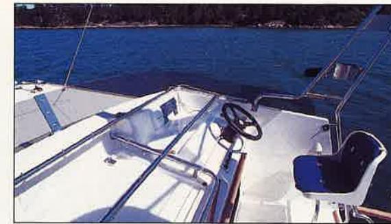
Left: boarding at the bow? A handy rail can be lowered for use as a footfall. Right: cruising under low bridges? The stainless steel radar gantry will hinge down to reduce the boat's air draught to 10ft 6in.
