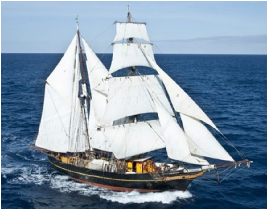
The engineless modern cargo transport sailing ship Tres Hombres. Image courtesy of Fair Transport.
