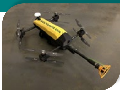
The Drone Thickness Gauge Multigaue 6000
