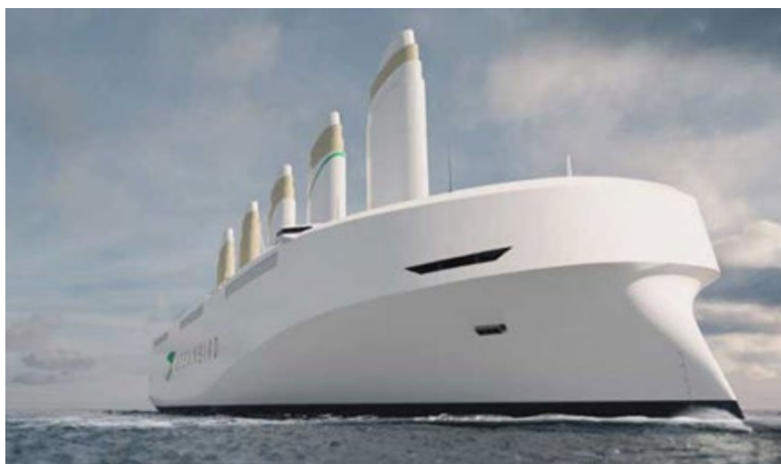
Wallenius Marine is developing the Oceanbird, able to ship 7,000 cars and trucks across the Atlantic propelled only by high-tech wing sails. Image courtesy of Wallenius Marine.
