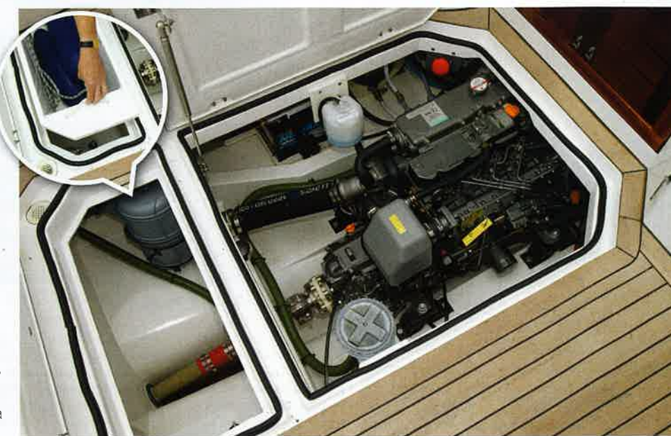
The large gas-strut supported hatch gives good engine access, and there's also room for a storage tray
