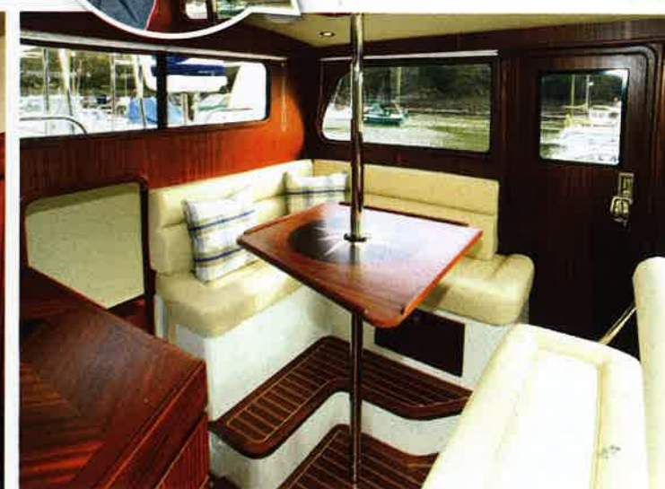
The helm seat backrest flips over to face the compact but pleasant dinette
