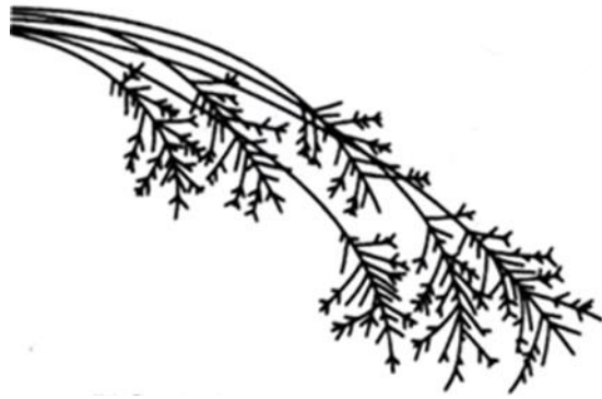
(b) Sparks from AISI 1045 steel (0.45wt.% Carbon)
