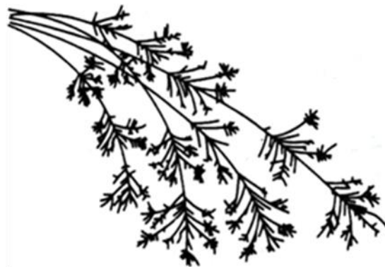
(c) Sparks from AISI 1095 steel (1.0wt.% Carbon)
