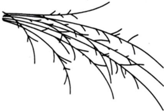
(a) Sparks from AISI 1015 steel (0.15wt.% Carbon)
