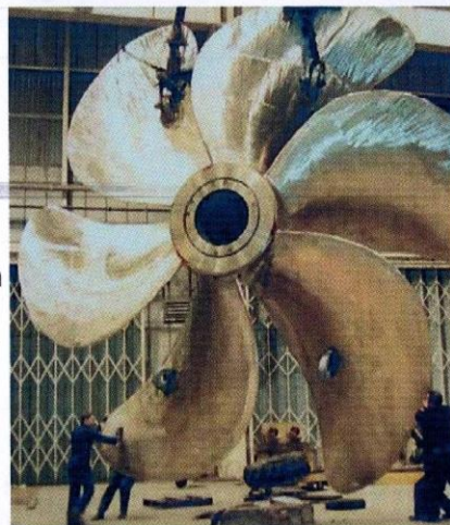
Nickel-Aluminium bronze ship propeller Courtesy Stone Marine Propulsion
