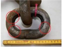
A chain link used in the lifting equipment of a fishing vessel showing fractures identified durina inspection
