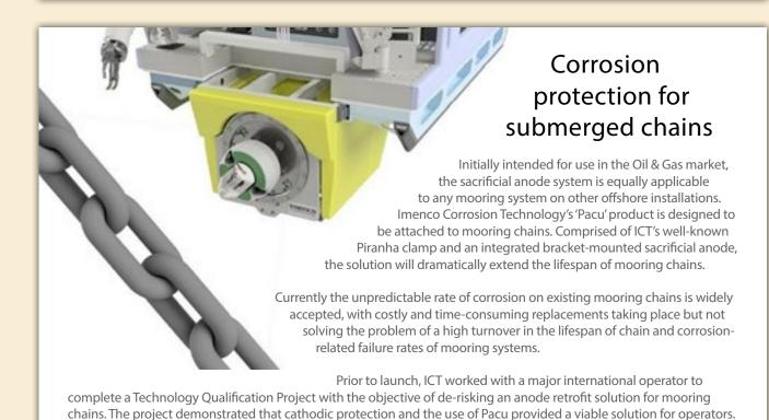
The use of Pacu will reduce the risk of mooring system failures while providing a cost-effective solution, which can be easily retrofitted to existing chains. The cathodic protection of chains opens up the opportunity to reduce corrosion allowances, thereby enabling thinner chains to be used in new and replacement systems. This leads to less weight and therefore less equipment needed for handling, transportation, and installation, reducing the carbon footprint of operations.
