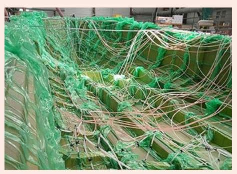
The hull of the new 26m Fly 86/2600 is the largest to date to be produced using Sicomin's GreenPoxy bio-epoxy system. "Our InfuGreen 810 resin really does offer the optimum solution for infusion in a large structure such as the Fly 86/2600," said Philippe Gruaud, head of technical sales for western France, Sicomin.
