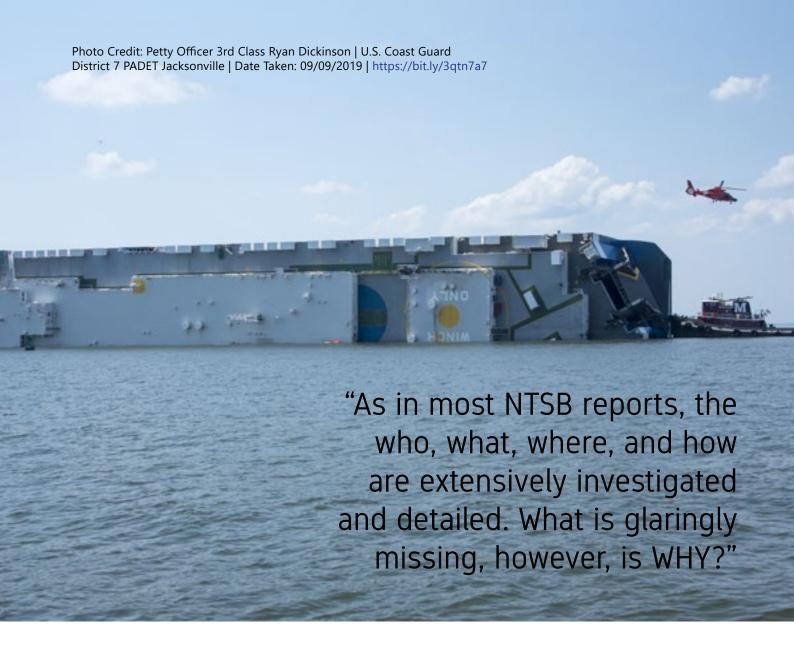
vessel in the final turn toward the open sea as the vessel sped up, it resulted in the centers of gravity and buoyancy rolling the vessel when she heeled past 8 degrees.
