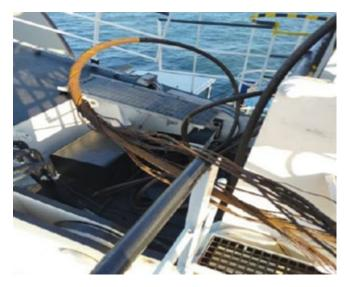
A concrete mattress was being deployed as part of the construction of a pipeline crossing. As the load was swung outboard and before it entered the water, the crane wire parted causing the load to fall to the seabed. The vessel was in a safe handling zone more than 5m from subsea assets. The mattress was overboarded when the crane was 17m from the nearest subsea asset.
