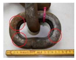
A chain link used in the lifting equipment of a fishing vessel showing fractures identified during inspection
