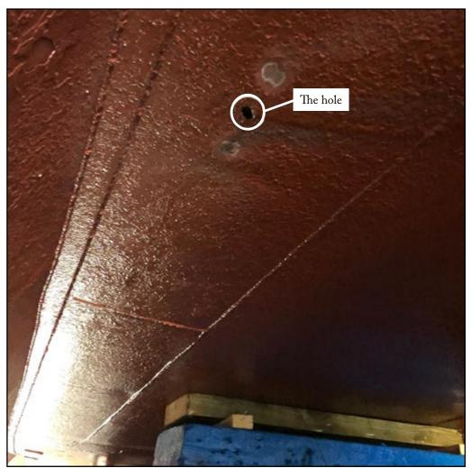
Figure: The 25mm hole in the fishing vessel's shell plating, observed when the vessel was lifted out of the water.
