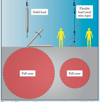
Figure 1: Illustration of the danger zone under a suspended load
