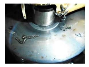
adjustments had been carried out. When removing the cylinder cover, small metal particles and partial destruction of the exhaust valve tappet tip was found. The evidence available indicated that the locking nut of the adjusting screw from the exhaust rocker arm (that regulates the clearance of the exhaust valve) had become loose. The most likely cause of this is that when reassembling, the locking nut had not been tightened as per the manufacturer's requirements.
