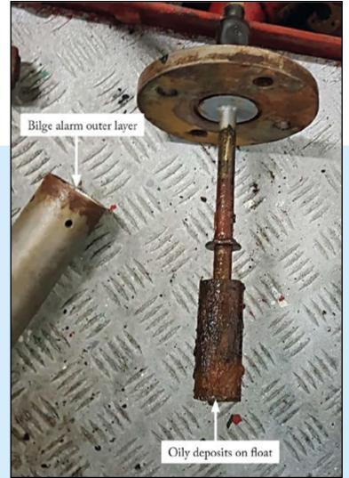
Figure 2: The disassembled bilge alarm, showing the build up of oily deposits on the float
