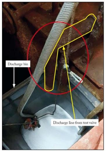
Figure 1: The discharge line from the test valve into the bin
