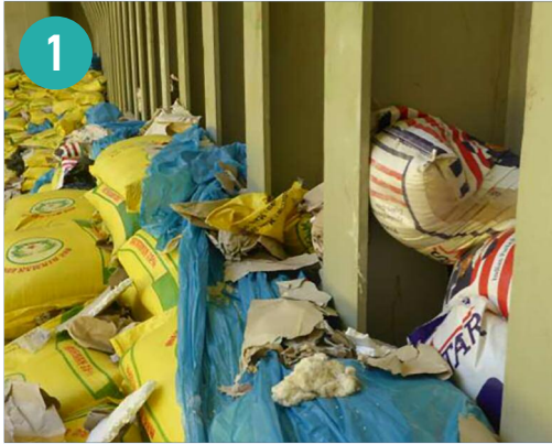
Figure 1: Example of dunnage materials at discharge. Bags shifted during the voyage dislodged dunnage materials between frames.
