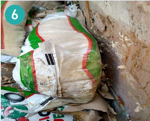
Figure 6: Example of mould damaged bag stowed against steelwork.
