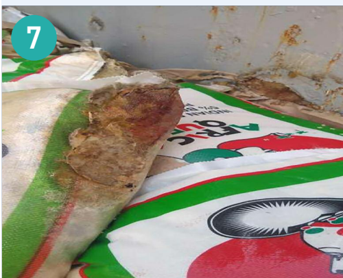
Figure 7: Example of damaged bag with mould growth and staining consistent with stowage against steelwork.
