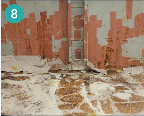
Figure 8: Example of bag / water staining of kraft paper on the tank top during discharge.
