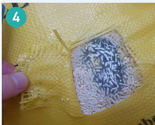
Figure 4: Mould growth beneath the packaging. Reproduced with kind permission of CWA
