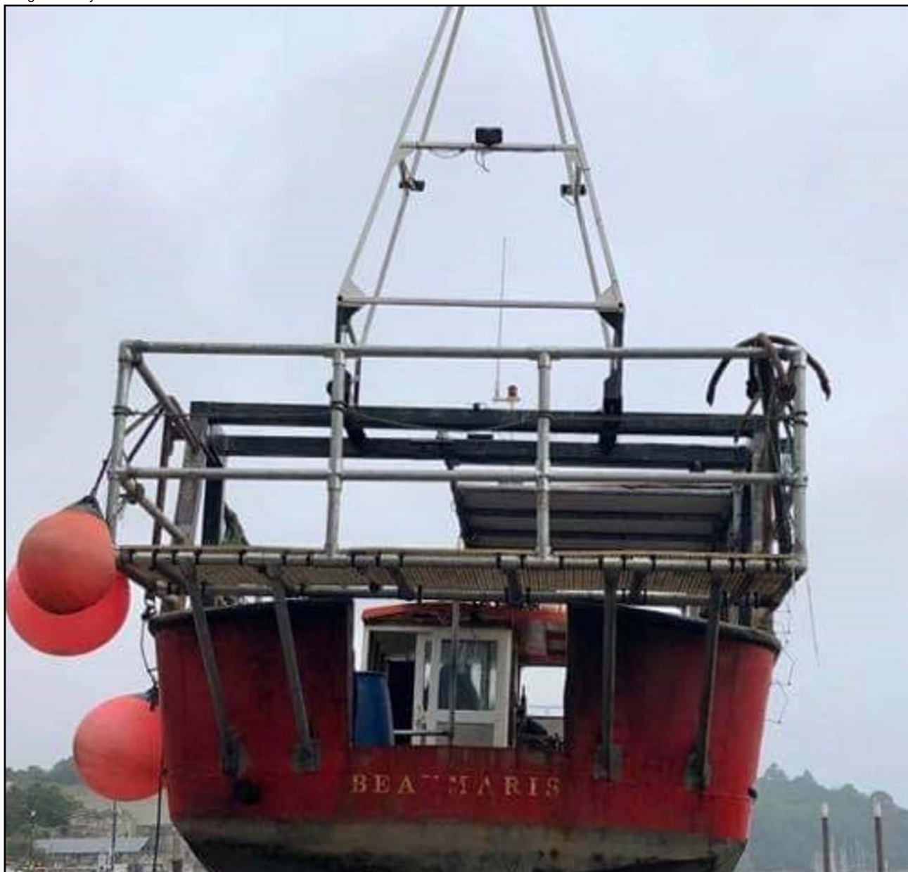
Figure 7: Large cat catcher fitted to Nicola Faith's stern
