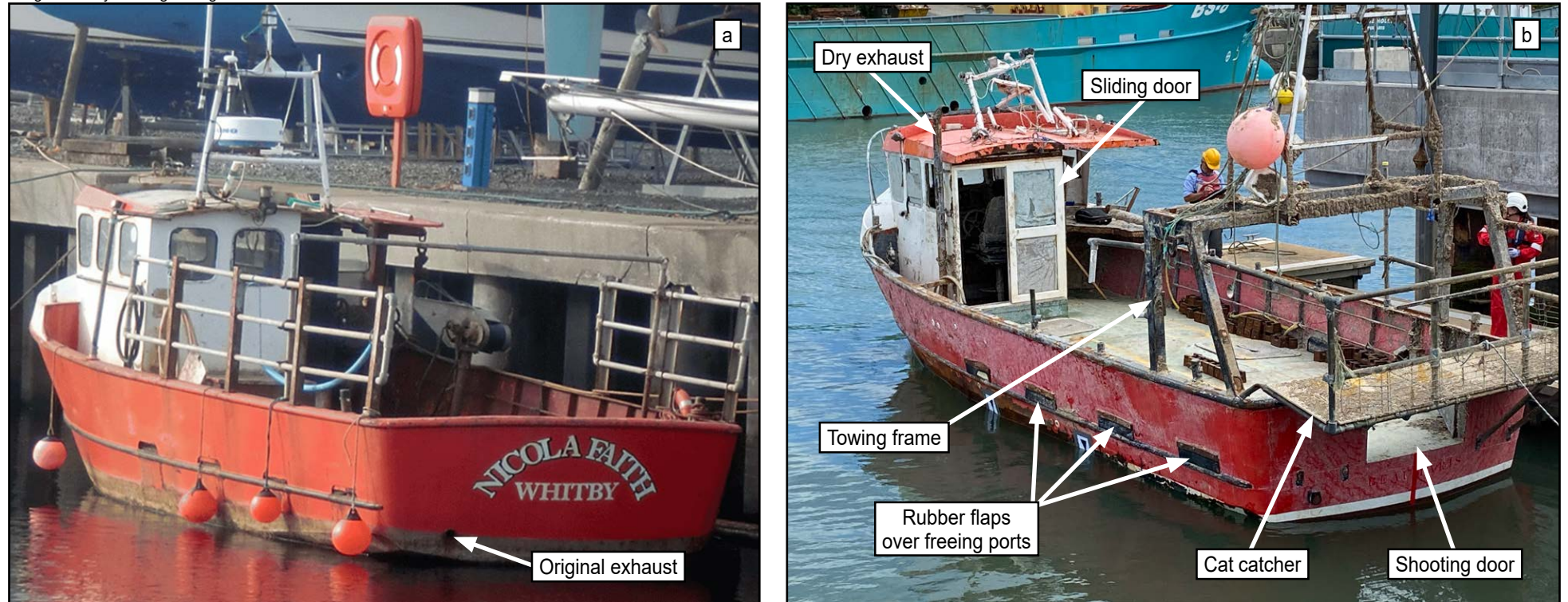
Figure 5: Nicola Faith as it was built, before any significant modifications (a) and Nicola Faith 's recovered wreck, showing modifications (b)
