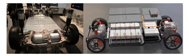
Figure 3 - Examples of the positioning of the battery packs in EVs, which is found in the chassis..
